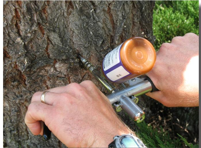
Injection System Without Drilled Holes
